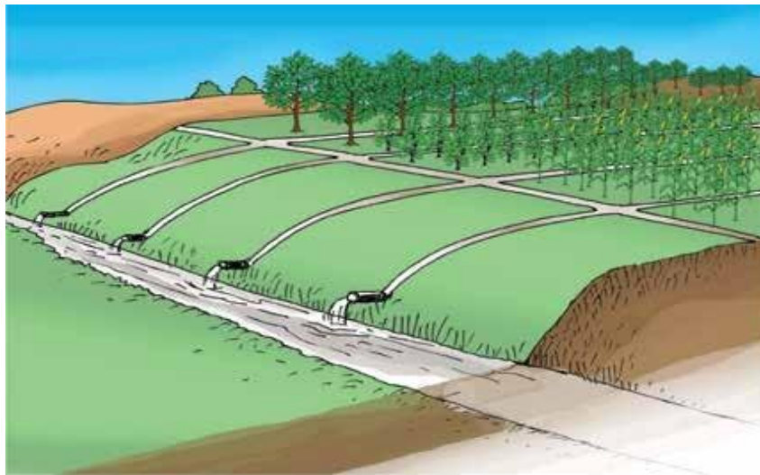
Figure 6.21 Drainage Channel (Source: Godinho et al. , 2023)
